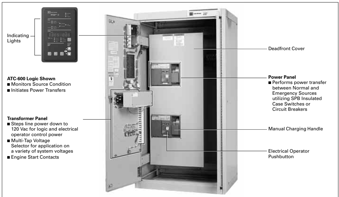
Figure 4. Basic Switch Components of SPB Automatic Transfer Switches
